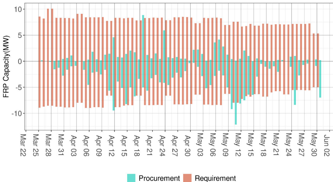
Figure 7: Daily Average requirement and procurement of upward and downward flexible ramping in the FMM for the TIDC BAA
